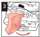
Rotate the recline foot to the back of the restraint and lock into place.
